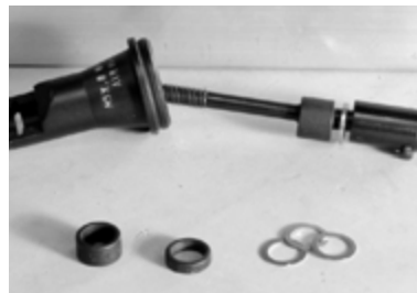
Front end assembly with longest spacer to suit 1.0D insert and shim washer.
